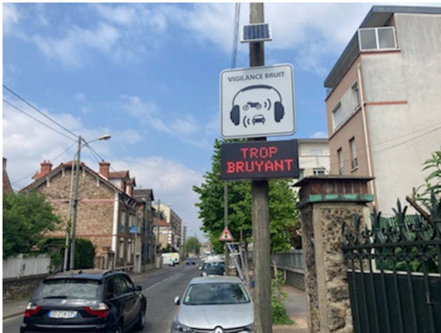
Figure 6: Educational noise radar designed by Bruitparif and installed in Juvisy-sur-Orge in France
