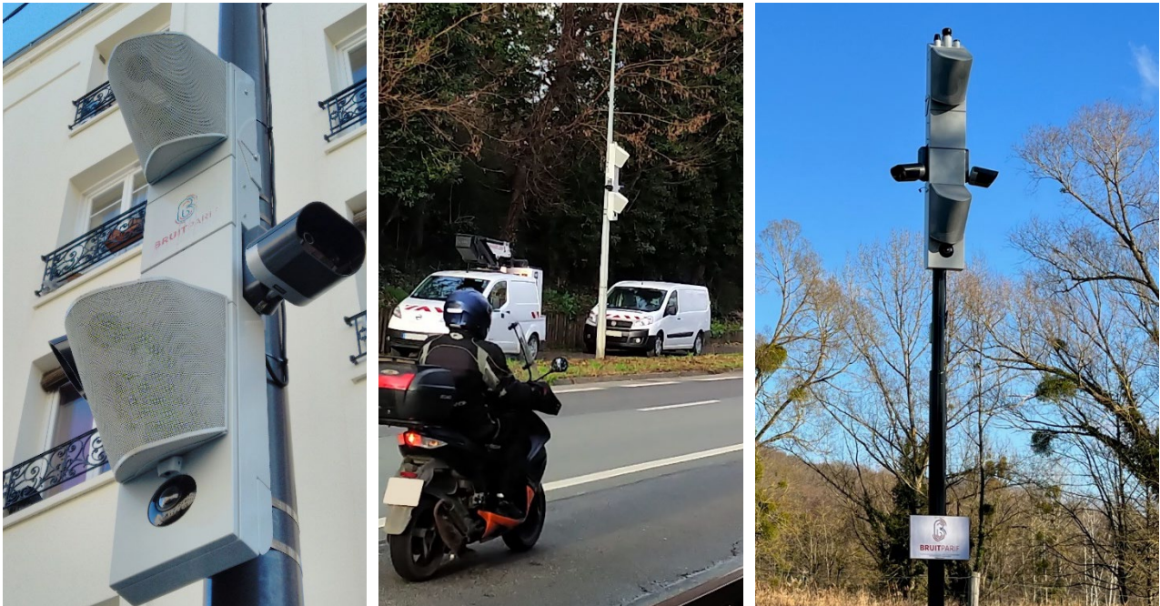
Figure 1: The noise radar prototype developed by Bruitparif installed in three of the pilot sites in Paris (on the left), in Villeneuve-le-Roi (in the center) and in Vallée de Chevreuse (on the right)
